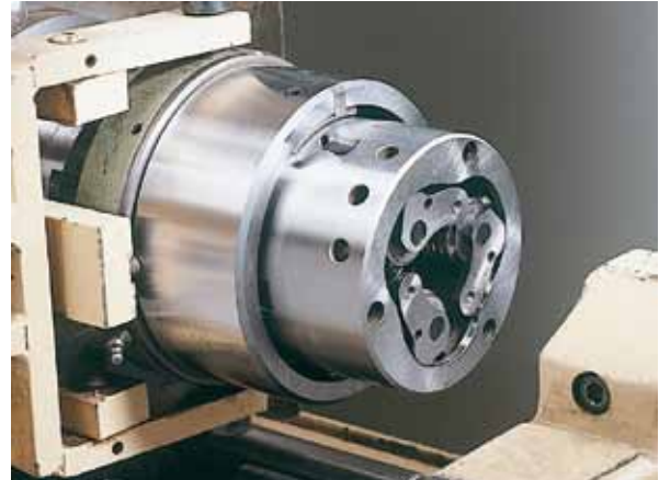
Rotary RR 22-2 rolling head mounted on a slide unit spindle
