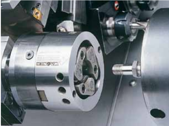
Stationary RS16 rolling head fitted on the turret of a CNC lathe
