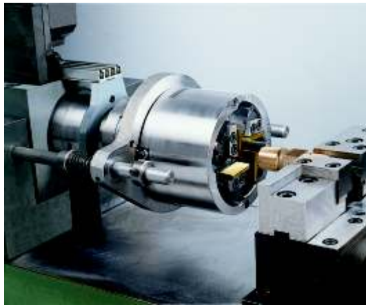
Centresleeve unit with cutting head Z 27 GK
