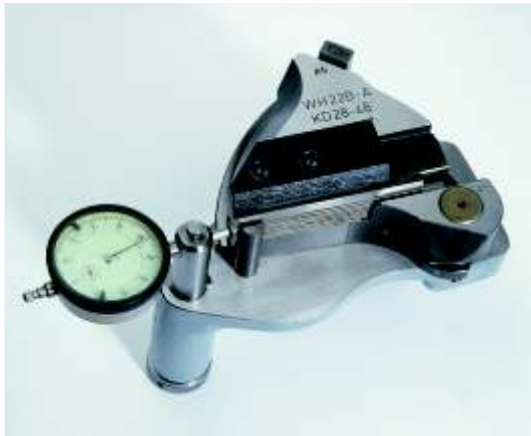
Setting the chaser in the chaser holder with the help of the setting device.
