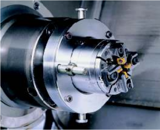
MSD 20 - R built up on a special purpose machine
