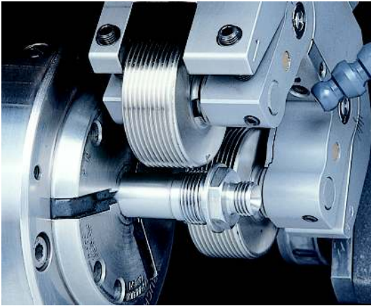
Thread rolling close to a collar.
